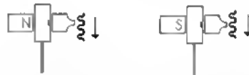
With the north pole at the back of the sensor absence of ferrous metal is sensed. With the south pole at the back of the sensor presence of ferrous metal is sensed. The sensor will normally need to be very close to the gear teeth.
